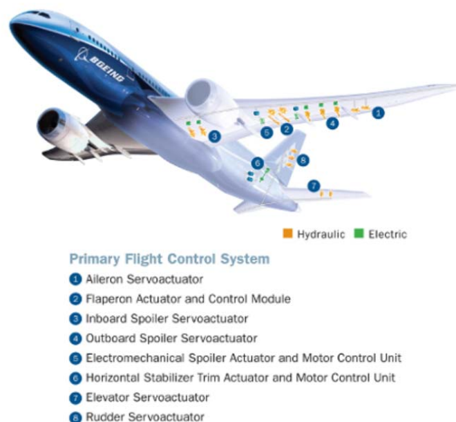
Figure 7: Primary Flight Control Systems
