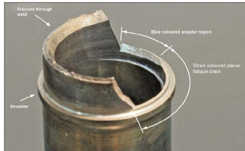
Figure 43: Oil feed stub pipe fracture
