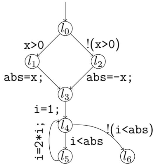
On the board: Shortest and longest program path starting in state  $(l_0, \sigma)$  with  $\sigma : \text{abs} \mapsto 2; i \mapsto 0; x \mapsto -2$
