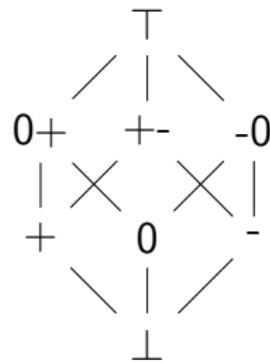
$$\begin{array}{llll} \llbracket T \rrbracket = \mathbb{Z} & \llbracket + \rrbracket = \mathbb{N}^+ & \llbracket - \rrbracket = \mathbb{Z} \setminus \mathbb{N}_0^+ & \llbracket 0 \rrbracket = \{0\} \\ \llbracket + - \rrbracket = \mathbb{Z} \setminus \{0\} & \llbracket 0 + \rrbracket = \mathbb{N}_0^+ & \llbracket - 0 \rrbracket = \mathbb{Z} \setminus \mathbb{N}^+ & \llbracket \perp \rrbracket = \emptyset \end{array}$$
