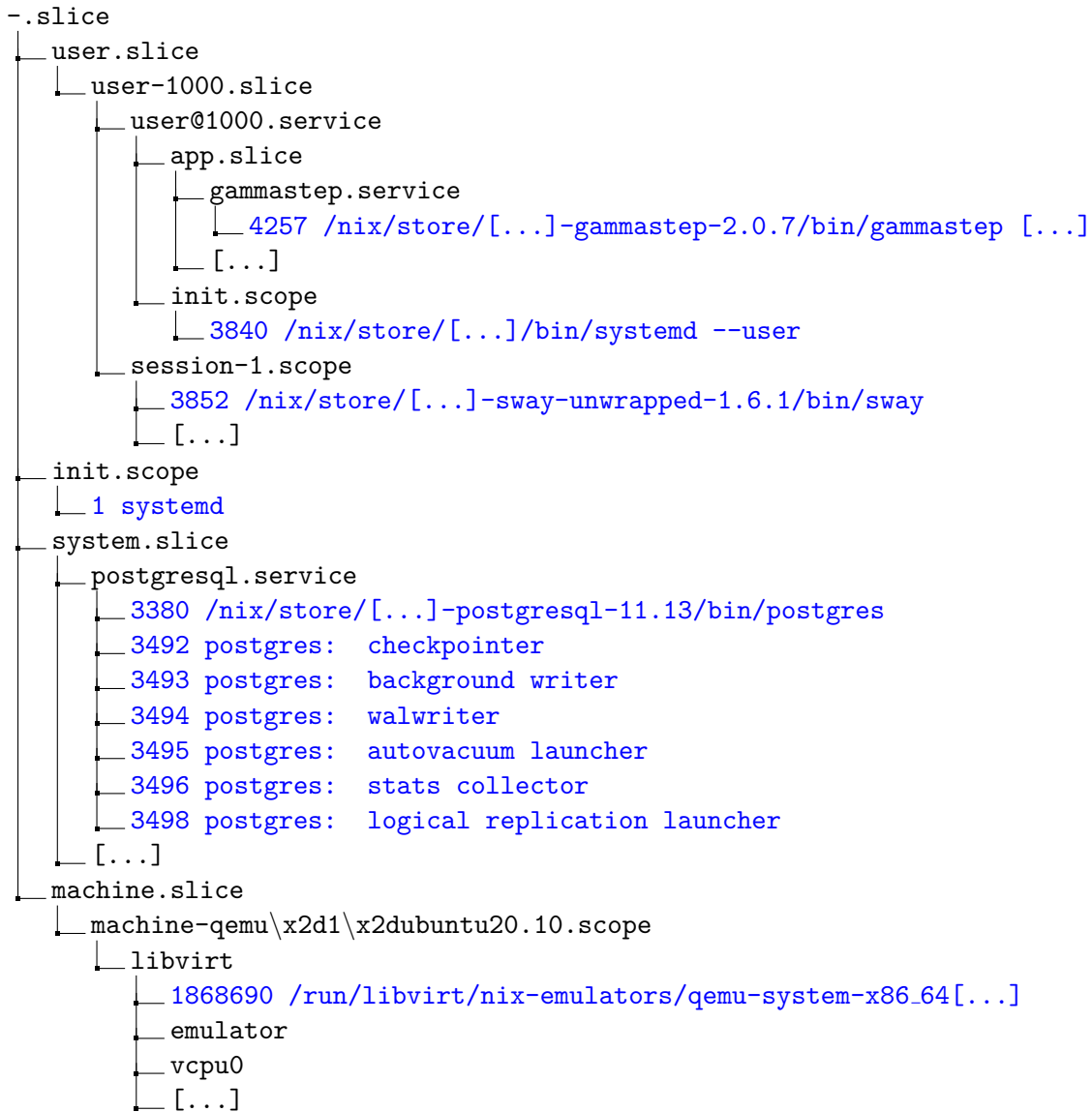
Figure 2.6: Shortened systemd cgroup hierarchy cgroups are shown in black, processes in blue
