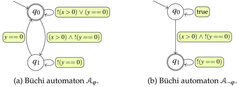
Figure 3.3: Fig. (a) on the left shows a Büchi automaton  $\mathcal{A}_1$  for the LTL-property  $\varphi = \Box(x > 0 \Rightarrow \Diamond(y = 0))$ . In this graph, the state  $q_0$  is both the initial- and accepting state. In comparison, Fig. (b) on the right shows a Büchi automaton  $\mathcal{A}_2$  for the negated LTL property  $\neg\varphi$ . The accepting state is  $q_1$ , and is simultaneously a sink state.
