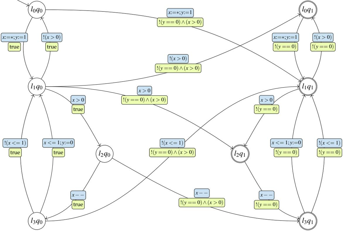
Figure 3.4: The Büchi Program  $\mathcal{B}$  is built from the product of the CFA that represents the input program  $\mathcal{P}$  (cf. Fig. 3.2b) and the Büchi automaton  $\mathcal{B}$  with the property  $\neg\varphi$  (cf. Fig. 3.3b).
