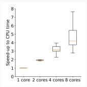
The ratio of the CPU time compared to the response time for 1, 2, 4, and 8 cores.
