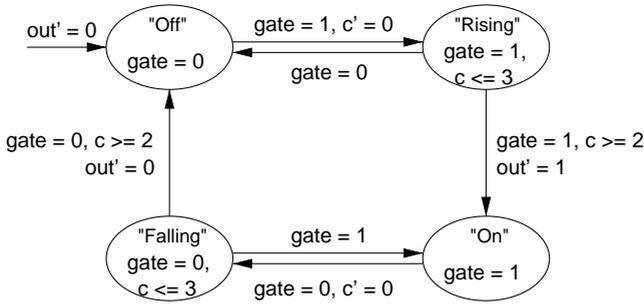
Fig. 1. Timed automaton for an nMOS transistor.
