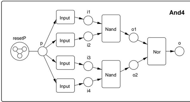
**Fig. 3.** Model of the AND circuit.
