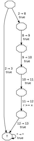
**Figure 4: Control-flow automaton for the example program with non-linear safety condition (cf. Fig. 3)**
